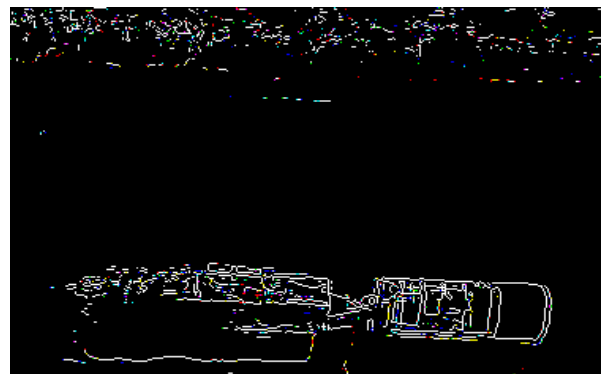
Fig. 7. The segmented original image without the influence of additive Gaussian noise ( \sigma_{\text{noise}}=0 ) using a method based on the Sobel filter
