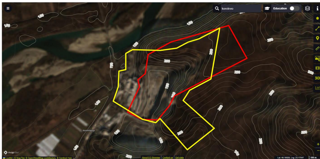
Fig. 1. Topographical plan of the project for the development and reclamation of the Korolivske andesite deposit in Berehove district, Zakarpattia region
