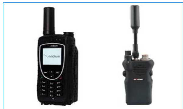
Fig. 7. Iridium and L3 Harris end devices for use in Iridium Tactical Communication System [13]
