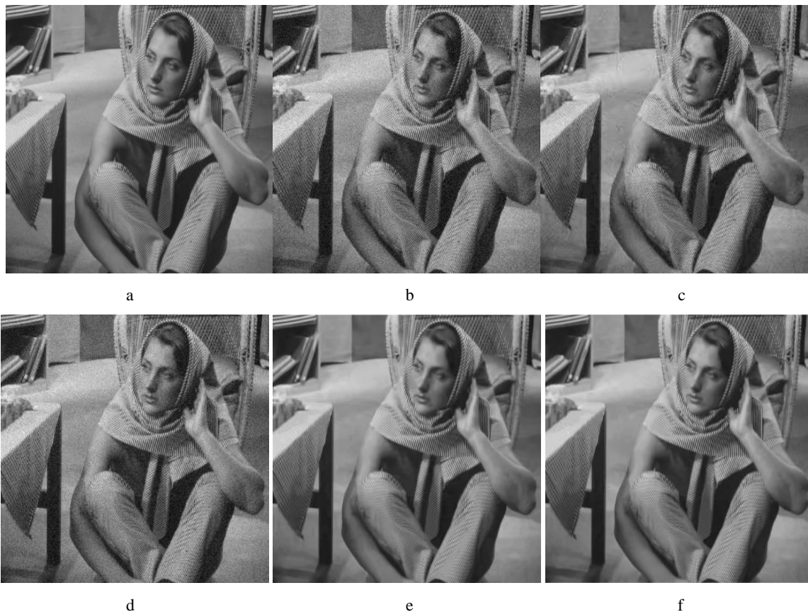
Fig. 7. An example of the original image (a), distorted by noise (b), compressed with losses at Q \approx Q_{OOP} (c), compressed with losses at Q \approx Q_{OOP} - 5 (d), filtering result for Q \approx Q_{OOP} (e) and filtering result for Q \approx Q_{OOP} - 5 (f)
