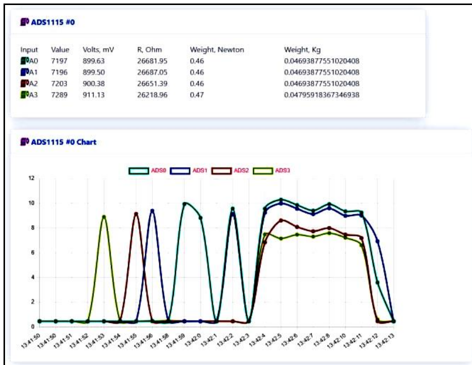
Fig 7. The result of the foot weight/pressure measurement, available to the doctor for analysis
